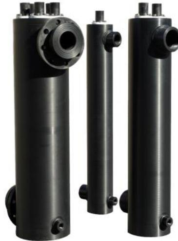
The UV reactor is made in HDPE - high density polyethylene material. This is the best material for corrosive liquids and sea water, as the HDPE is UV-stabilised. Thanks to special welding procedures the UV chamber can be used up to a max pressure of 6 bars. The reactors have a horizontal or vertical position depending on the model.
