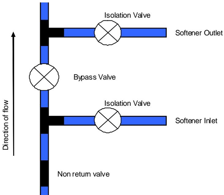
**Typical bypass setup using three isolation valves plus a non return valve.**
